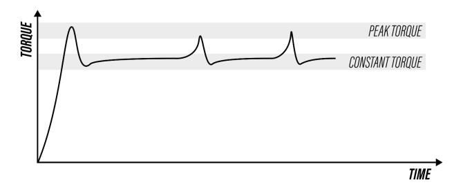
Most people visualize the strength of the motor as the strength their own arms must deliver in a long corner, which could compare to how many g's you would take in a corner in a real car. This vision of motor power is close to the definition of constant torque. The constant torque is the power the motor can maintain in the long run, after hours of racing.
