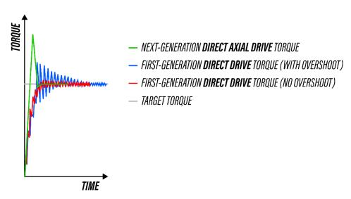
This is a comparison between an overshoot of our Direct Axial Drive wheel base, and First-Generation wheel bases from our competitors. You can see that controlled overshoot stabilizes the motor's performance far more quickly back to the motor's target torque, as it uses less unnatural counterforces to correct itself.
